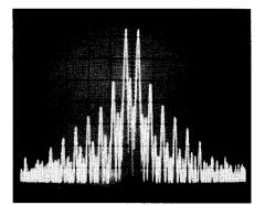
Fig 1—Spectral display of the TS-50S transmitter during two-tone intermodulation distortion (IMD) testing. Third-order products are approximately 30 dB below PEP output, and fifth-order products are approximately 42 dB down. Vertical divisions are 10 dB; horizontal divisions are 2 kHz. The transceiver was being operated at 100 W PEP output at 14.2 MHz.
